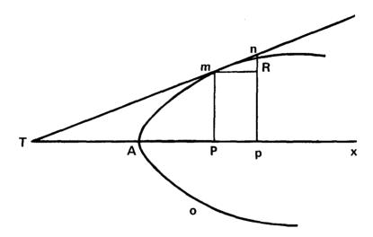
Assume that the line nAo is any curve whose nature (whether it's a parabola, ellipse, etc.) is *unknown* to us and on which a tangent is to be drawn at point m.
